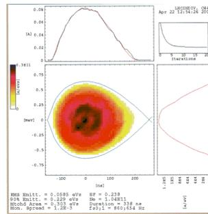
Fig. 1: Tomographic reconstruction of the individual bunch LHC beam in the PSB at the end of step 2 (Fig. 2): intensity  $\sim 1 \times 10^{11}$ , longitudinal emittance  $\sim 0.3$  eVs.
