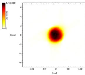
Fig. 3: Tomographic image of the LHC Probe beam in the PSB; intensity  $5.2 \times 10^9$  protons, momentum spread  $\sim 10^{-3}$ , bunch length  $\sim 70$  ns and longitudinal emittance  $\sim 0.2$  eVs.
