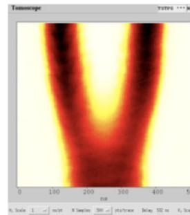
Fig. 5: Bunch splitting of the 50 ns-type LHC beam in PSB ring 3.
