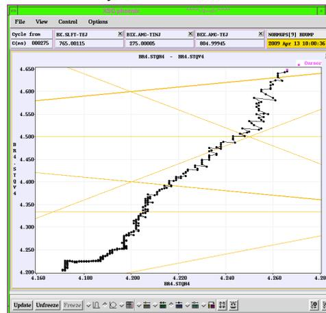
Figure 2: Dynamic tune diagram of ring 4 along the cycle.
