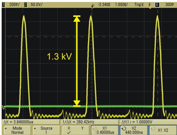
Figure 9: Pulse with 1.3 kV at 260 kHz repetition rate for first stacking stage.
