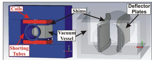
Figure 3: Magnetic dipole and electric deflector layout.
