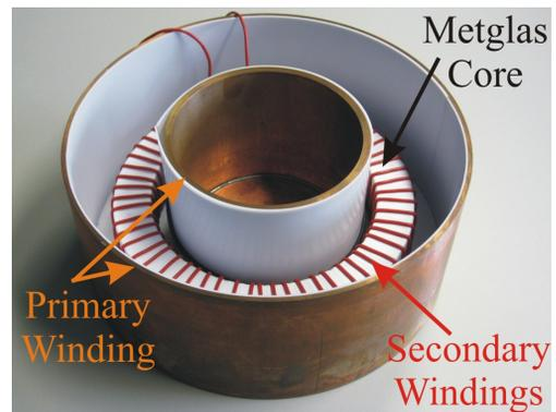
Figure 7: Nanocrystalline Tape Wound Transformer Core.
