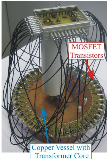
Figure 8: Parallel transistor array for fast kicker.
