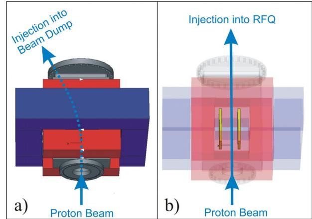
Figure 2: E×B chopper system: The static magnetic deflection (a) is compensated during a short pulse by an electric field between deflector plates inside the dipole gap (b).
