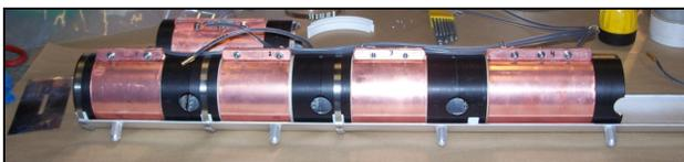
Figure 3. New FEPS module prior to installation.
