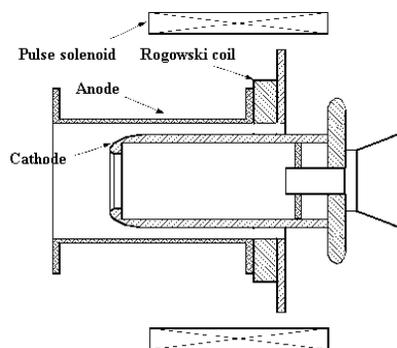
Figure 2: The gun design for nanosecond mode.
