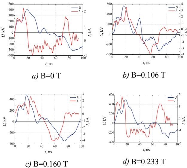
Figure 5: Synchronous oscilloscope plots of the gun current and voltage at different values of magnetic field  $B$ . The charge voltage of the Marx generator was 32 kV.
