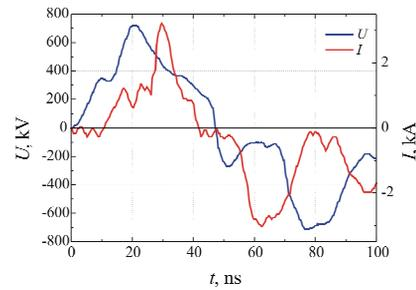
Figure 6: Oscilloscope plots of the gun current and voltage at a magnetic field  $B=0.266$  T. The charge voltage of the Marx generator was 40 kV.
