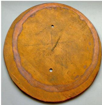
Figure 4: Ring beam track on a copper target with diameter 140 mm at the microsecond output.
