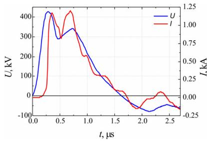
Figure 3: Beam current and gun voltage at magnetic field  $B=0.34$  T at the microsecond output.
