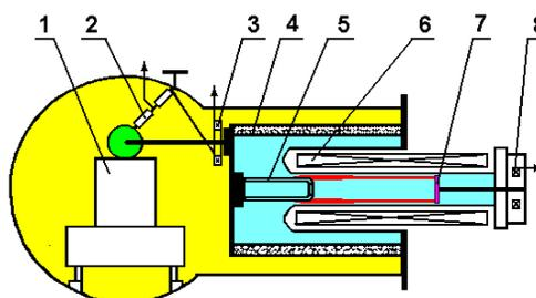
Figure 1: Scheme of the microsecond output with SEMIG. The electron beam is marked by red. 1 – 8-stage Marx generator; 2 - voltage divider; 3 - Rogowski coil for total current measurement; 4 - insulator; 5 - cathode; 6 - solenoid; 7 - collector with copper target; 8 - Rogowski coil for beam current measurement.
