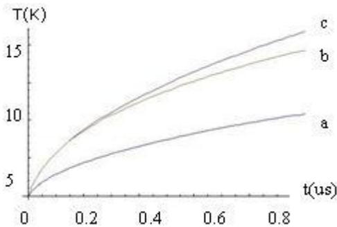
Figure 4: Line (a) is the temperature rise vs time for the infinite plane surface; Line (b) is the temperature rise at the crack upper corners; Line (c) is the doubled Line (a).
