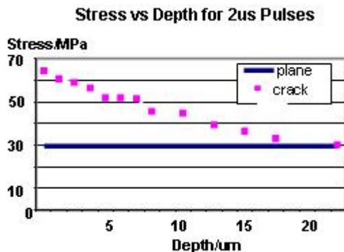
Figure 8: Stress vs crack depth at 2μs pulses.
