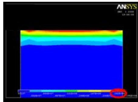
Figure 6: Contour plot of von Mises stress on the smooth metallic plane.
