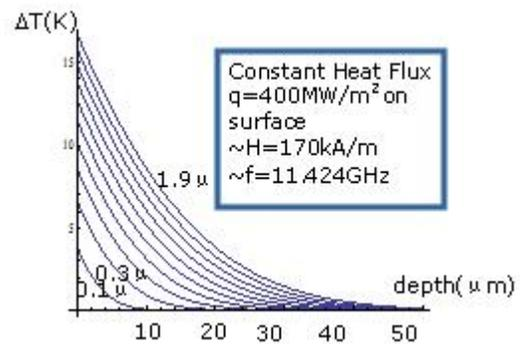
Figure 2: Elevated temperature profiles at ten time intervals, for a smooth, uncracked metallic surface.
