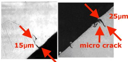
Figure 1: Cracks in accelerating structure (reproduced from Ref. [5]).
