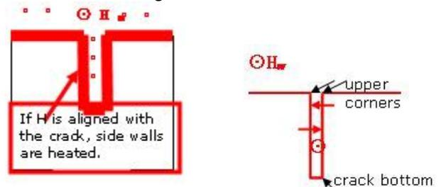
Figure 3 (a): Sketch of a structure with a crack. (b): Maximum temperature rise takes place at the upper corners of the crack.
