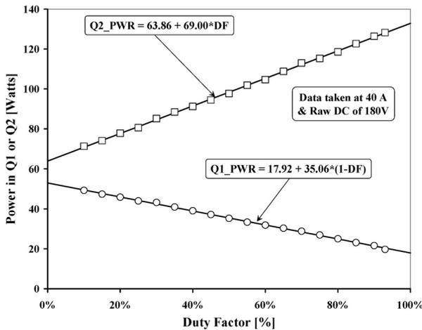
Figure 3: Q1 - Q2 total losses vs. duty factor.
