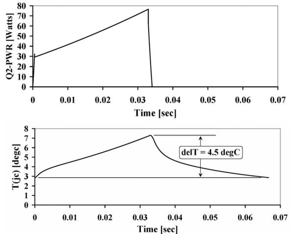
Figure 8: Q2 power and junction temperature.
