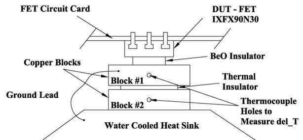
Figure 1: Thermal measurement setup.
