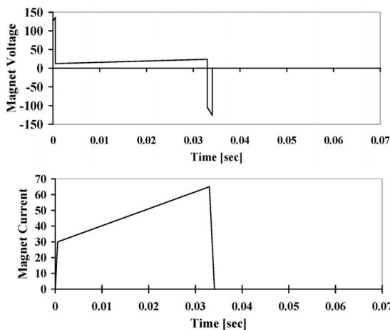
Figure 6: Voltage and current ramp for maximum temperature rise.
