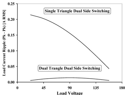
Figure 7: Load current ripple vs. output voltage.
