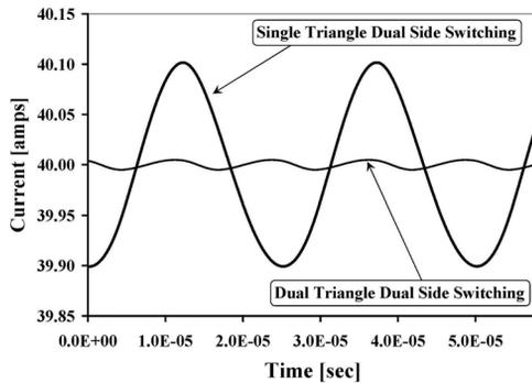
Figure 6: Output load current (at phase reference of 25%).
