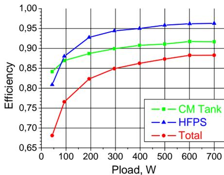
Figure 6: The tank, HFPS and the total efficiency dependence on the output power at Toshiba klystron dummy load.
