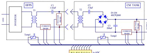
Figure 5: Connection module test run circuit.
