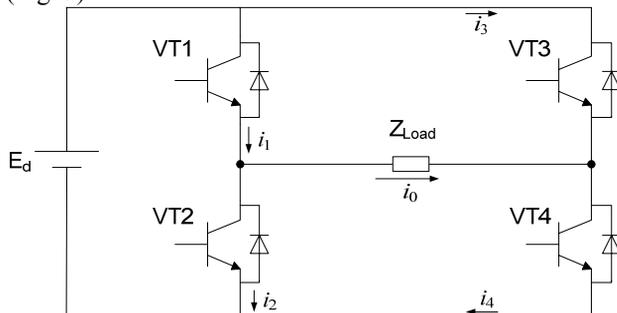
Figure 3: Phase-shifted pulse modulation inverter.
