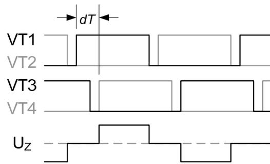
Figure 4: The duty cycle of PSM scheme.
