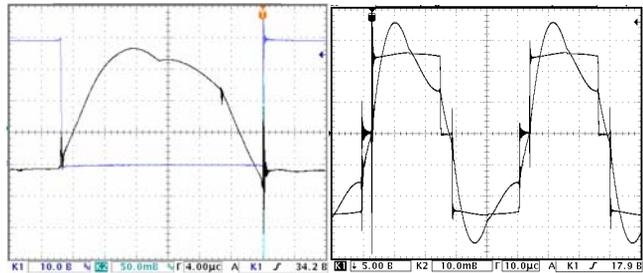
Figure 8: Left – Current and voltage through one of the inverter switches; Right – Interter output current and voltage.
