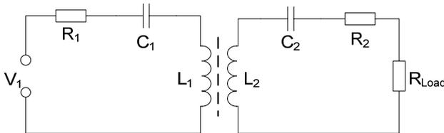
Figure 2: Resonance circuit of loosely coupled transformer.
