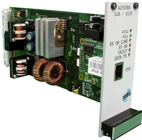
Figure 4: single board, 5 A bipolar power supply developed at Elettra (A2505).
