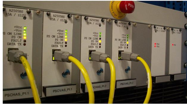
Figure 5: Crate containing 4 A2505 units with auxiliary “bulk” power supplies.
