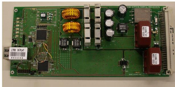
Figure 5: Prototype of the single-Board, 10 V/ 5A bipolar fully digitally controlled power supply designed at Elettra
