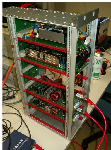
Figure 6: Prototype setup of a 4 channels sub-rack (two channels only are mounted and connected to the control)
