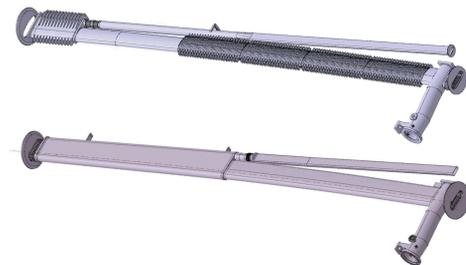
Figure 6: Old (top) and new (bottom) MU16 extraction vacuum chamber design.
