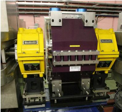
Figure 3: Picture of the SS39. The two yellow sextupoles are interleaved by the violet octupole.
