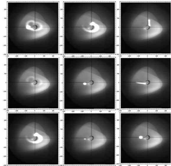
Figure 7: Various beam sweeps and sizes on the BTVDD.
