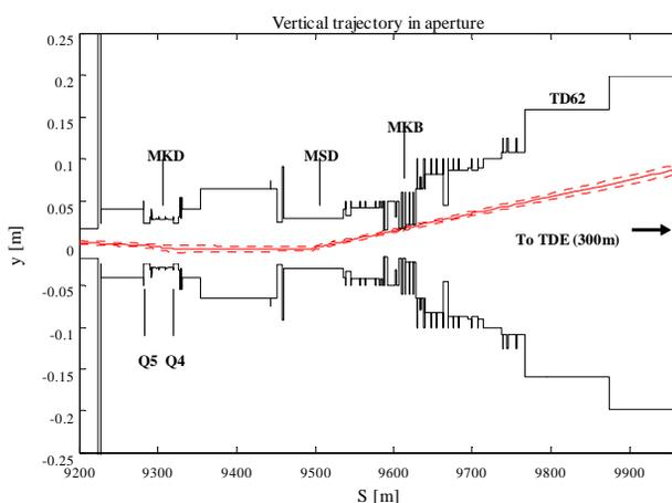
Figure 1: Vertical trajectory of first beam extracted into TD62. A  $\pm 3$  sigma envelope for nominal optics and measured emittance is shown. The aperture restriction 15 m before the MKB is the differential pumping section.
