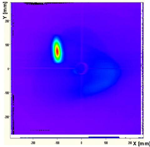
Figure 2: BTVDD image of first beam extracted to TDE 62 using extraction kickers. The visible beam spot is about 30 mm wide and 80 mm high.
