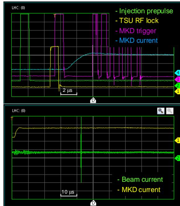
Figure 4: Synchronisation during “Inject and Dump”. The injection prepulse, PLL lock and initial MKD trigger are followed by multiple re-trigger signals. The extracted bunch is in the centre of the kicker waveform.
