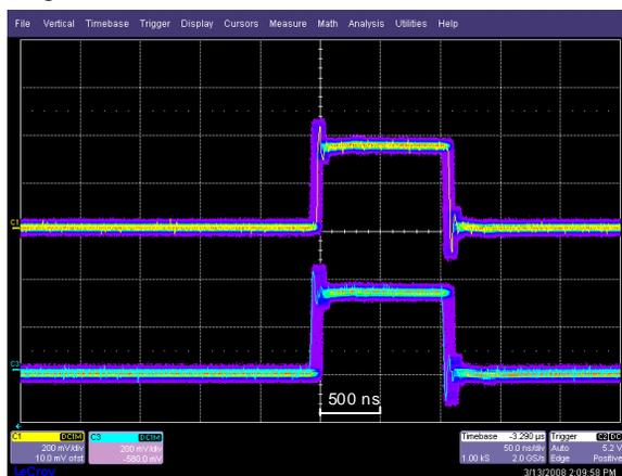
Figure 3: Locking of the two dump triggering and synchronisation unit PLLs to the RF revolution frequency.
