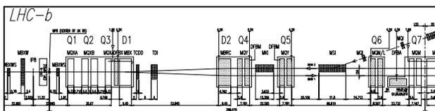
Figure 1: Schematic view of the Beam 2 injection.
