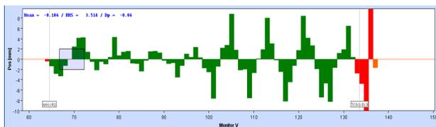
Figure 5: Injected beam trajectory during MKI flashover. The oscillation starts at the MKI and shows an overkick of about 5-6  $\sigma$  (the larger oscillations further downstream in the LHC are due to the measurements taking place at that time).
