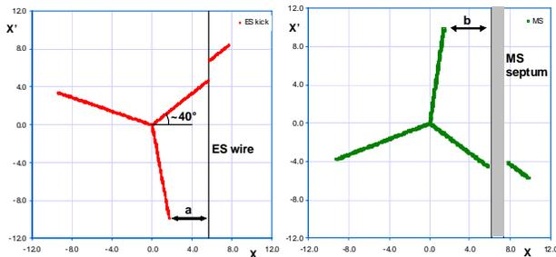
Figure 2: With a phase advance of  $78^\circ$  from ES to MS, the extracted separatrix should have an angle of about  $40^\circ$  with respect to the X axis, to optimise clearances **a** and **b**.
