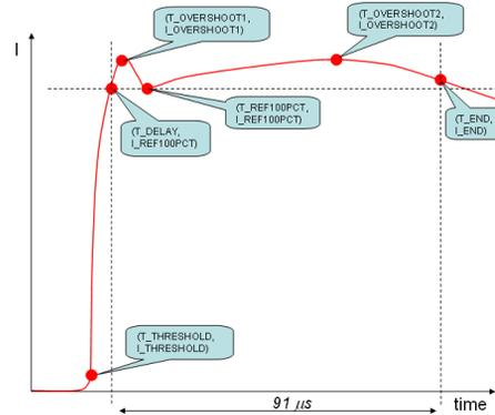
Figure 1: Description of the characteristic points of the extraction kicker current waveform.
