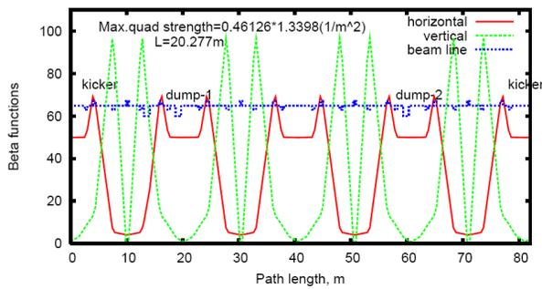
Figure 6: Optical design of Mu2e extinction channel. AC dipoles are indicated as “kickers” and the collimators as “dumps”.
