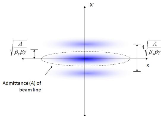
Figure 4: Effect of the AC dipole field in phase space. Beam line admittance  $A$  is indicated by the ellipse.
