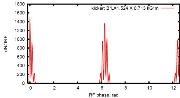
Figure 8: Time distribution of surviving beam, plotted as a function of the phase corresponding to the bunch frequency (twice the AC dipole phase). Pseudo-bunch separation is approximately 50 ns.
