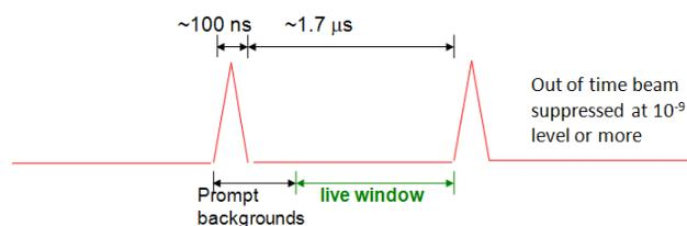
Figure 1: Proton bunch timing required by the Mu2e experiment.
