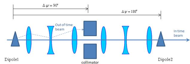
Figure 2: General scheme of the AC dipole extinction channel. Beam is only transmitted at times near the nodes of the AC dipole resonant circuit.
