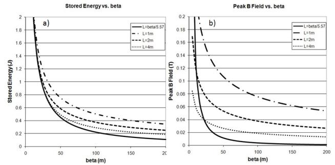
Figure 5: The dependence of peak stored energy (a) and peak magnetic field on  $\beta_x$  at the location of the AC dipole. Note that a length of  $L = \beta_x/5.57$  corresponds to the optimum length for a particular  $\beta_x$ , in terms of minimizing the total stored energy.
