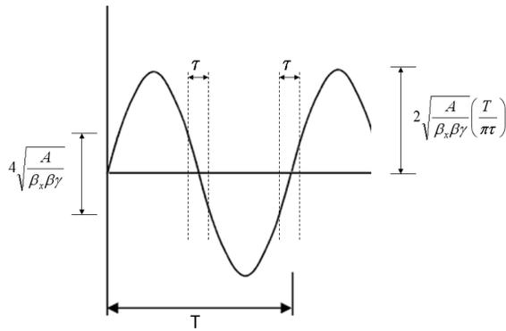
Figure 3: Concept for the AC dipole system. Because beam is transmitted at the node, the system only needs to run at half the bunch frequency. However, producing a short transmission window requires the system to run at a higher amplitude than would otherwise be needed.
