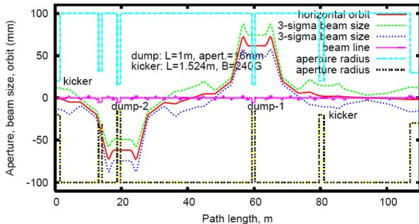
Figure 7: Trajectory of beam deflected by the first AC dipole, such that beam is fully extinguished. Three sigma envelope for a  $20\pi$ -mm-mr (95%) beam is shown.
