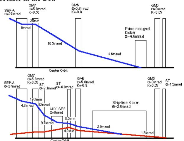
Figure 1: Trajectory of the beam extraction – Pulse magnet kicker (upper), strip-line kicker with bump orbit and auxiliary septum (lower). The red line in the lower figure is the local bump orbit.
