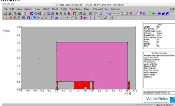
Figure 6: Cross section of the designed auxiliary septum.
