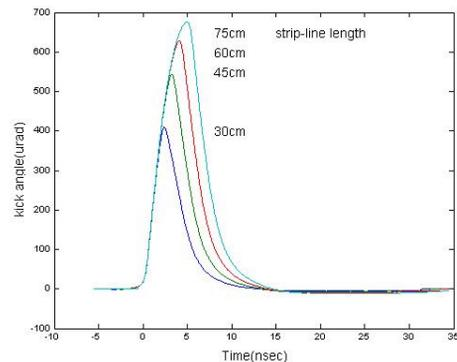
Figure 4: Calculation of the kick angle in the case of 30, 45, 60 and 75cm long strip-lines.
