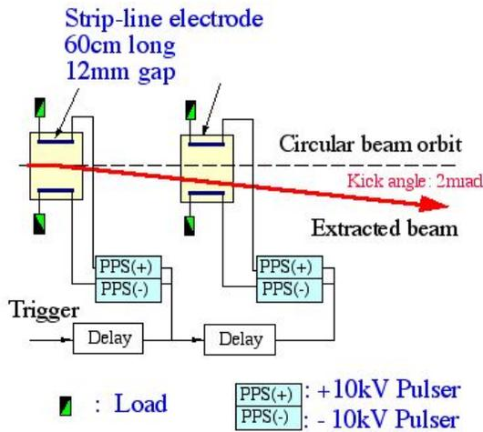
Figure 2: schematic layout of the strip-line kicker.
