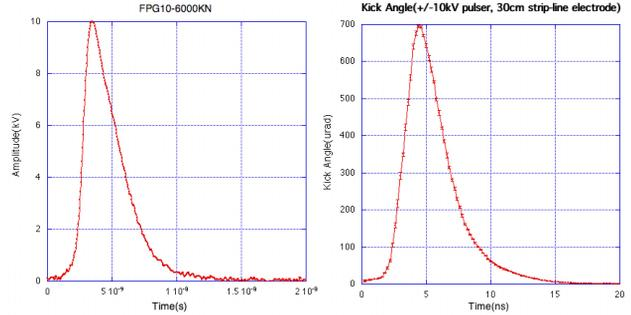
Figure 3a(left): Waveform of the FPG10-6000KN; Figure 3b(right): Beam kick profile using a pair of FPG10-6000KN and a 30 cm long strip-line kicker.
