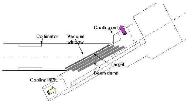
Figure 7: Targetry for the isotope production.
