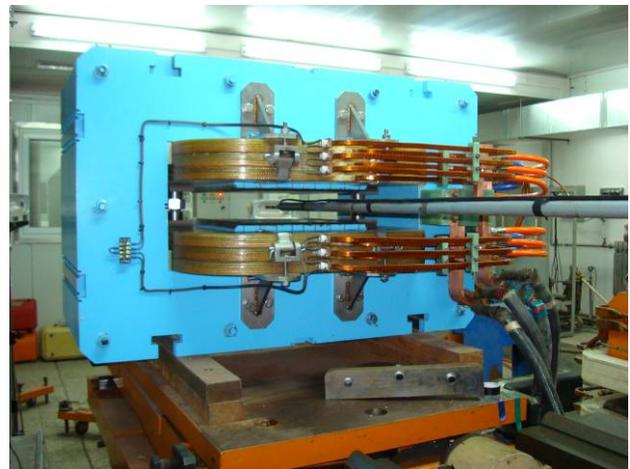
Figure 3: AC magnet for beam distribution.
