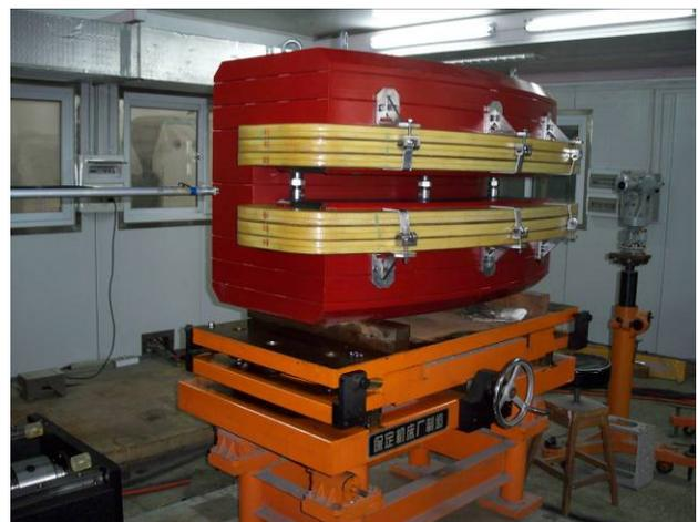
Figure 4: 45° dipole magnet.
