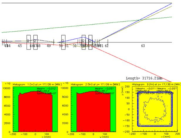
Figure 2: Beam optics of TR103 simulated with TRACE3D and TUTLE code.
