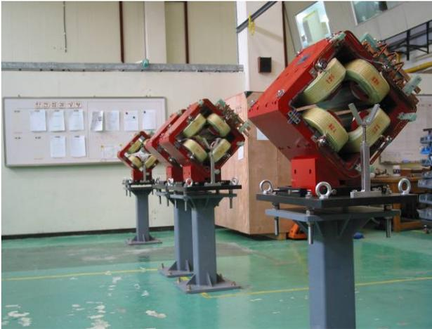
Figure 5: quadrupole magnets.
