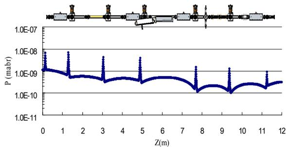
Figure 7: Pressure profile of the injection section at 3 GeV, 400 mA after a conditioning time of 100 A·h.
