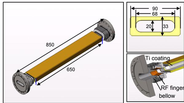
Figure 4: Configuration of TPS ceramic chamber.
