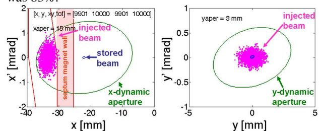
Figure 4: Simulated injected beam distribution, no BTS windows.
