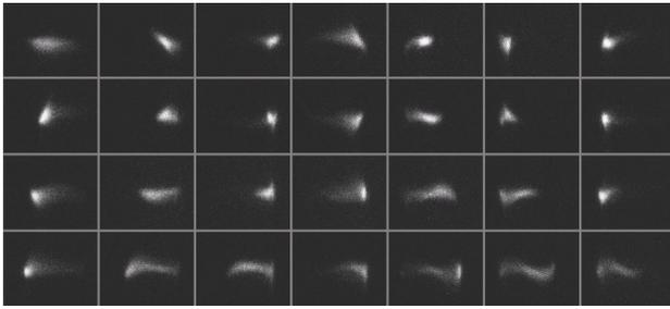
Figure 5: Single-turn injected beam profiles after removing the BTS vacuum windows.
