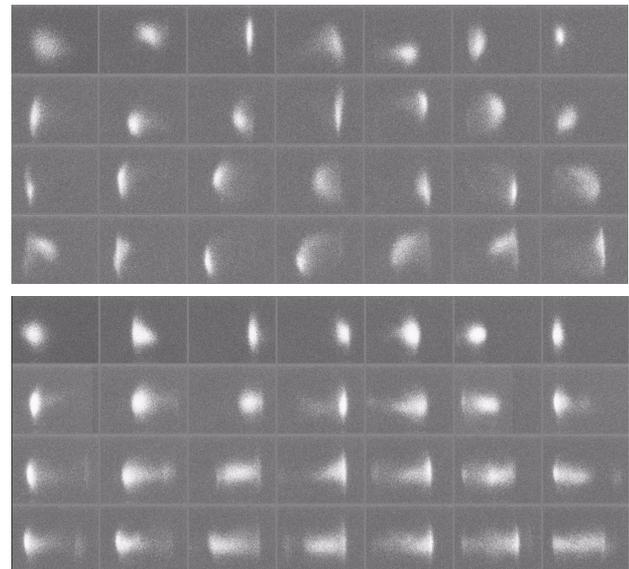
Figure 3: Synchrotron light monitor (SLM) measurements of the single-turn transverse profiles of the injected beam in SPEAR for the first 28 turns. Top: before BTS tuning. Bottom: after BTS trajectory and optics tuning.
