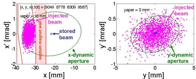
Figure 1: Simulated injected beam distribution.
