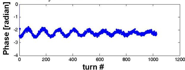
Figure 6: Measured synchrotron oscillations of injected beam in SPEAR.
