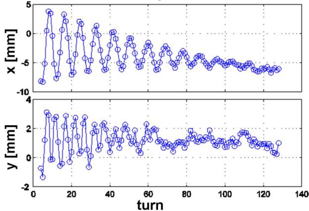
Figure 2: Measured betatron oscillations of the injected beam in SPEAR.
