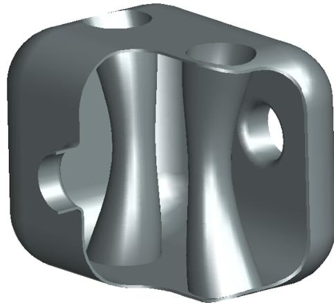
Figure 3: Conceptual design of a parallel-bar deflecting cavity.
