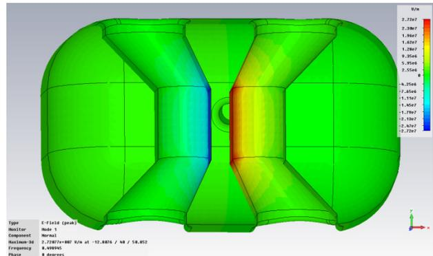
Figure 4: Preliminary design of a 499 MHz parallel-bar deflecting cavity.
