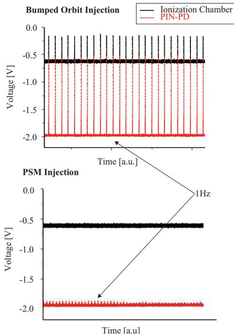
Figure 5: Stability of photon intensity at BL-14A in the pulsed bumped orbit injection (upper graph) and the PSM injection (lower graph). The spike appeared at exactly 1 Hz in both graphs. The horizontal scales are different in the two graphs.
