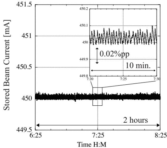
Figure 2: Stability of stored beam current during the top-up injection with the PSM.
