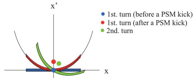
Figure 4: Schematic view of distributions and their centers of a stored beam in phase space. Blue, red, and green color strips show distributions of a stored beam just before and after a PSM kick and at the 2<sup>nd</sup> turn respectively. The corresponding color circles represent their beam centers.
