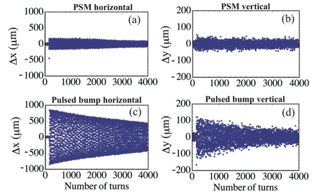
Figure 3: Horizontal and vertical beam oscillations ( $\Delta x$  and  $\Delta y$ ) of the stored beam immediately after the beam injection. The oscillations produced by the PSM injection are shown in the upper two figures, (a) and (b), and those by the bumped orbit injection are in the lower two figures, (c) and (d).
