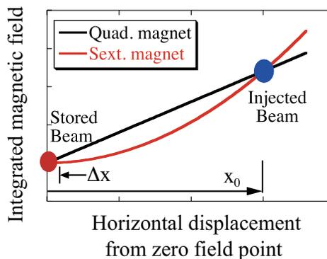
Figure 1: Integrated magnetic field of PSM and PQM as a function of the horizontal displacement from the zero field point. To compare effects of the two magnets on a stored beam, both magnets’ fields are drawn so as to have the same value at the position of an injected beam.
