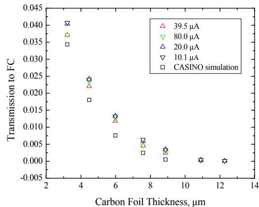
Figure 4: Measured (for different E-gun currents) and simulated by CASINO dependence of electron beam transmission to FC on carbon foil thickness.
