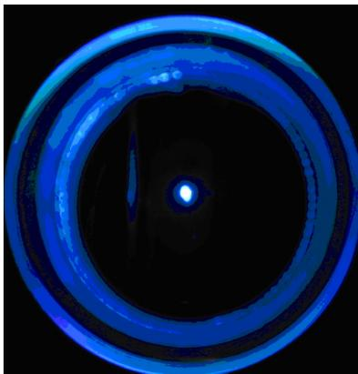
Figure 3: Image of focused electron beam on the P47 scintillator.
