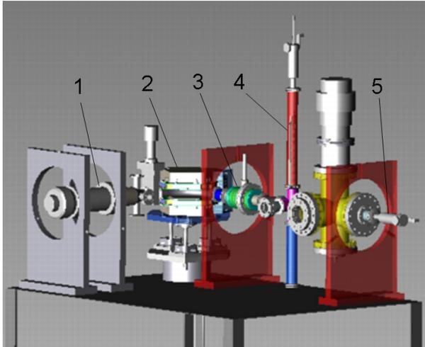
Figure 2: Low energy electron beam monitor: 1 – e-gun, 2 – bending magnet, 3 – electrostatic gridded lens, 4 – movable carbon foils and scintillator holder, 5 – movable Faraday cup.
