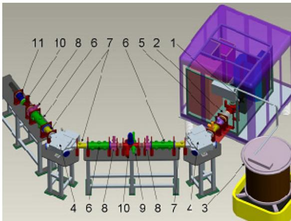
Figure 5: General view of the injector: 1- all permanent magnet ECRIS installed on HV platform, 2- 75-kV accelerating tube, 3- isolation transformer, 4- 60° bending magnet, 5- Einzel lens, 6- electrostatic triplet, 7- electrostatic steering plates, 8- rotating wire scanner, 9- horizontal slits, 10- Faraday cups, 11- emittance probe.
