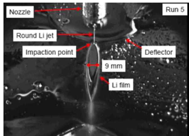
Figure 1: 9 mm wide liquid Li film flowing at about 58 m/s with thickness of about 10  $\mu\text{m}$ .
