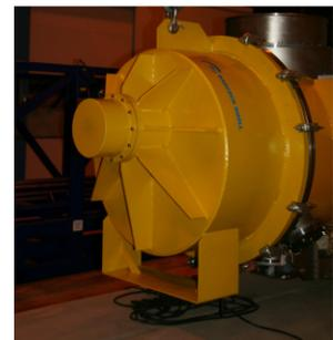
Figure 1: The damping frame, the coils and an end cap.
