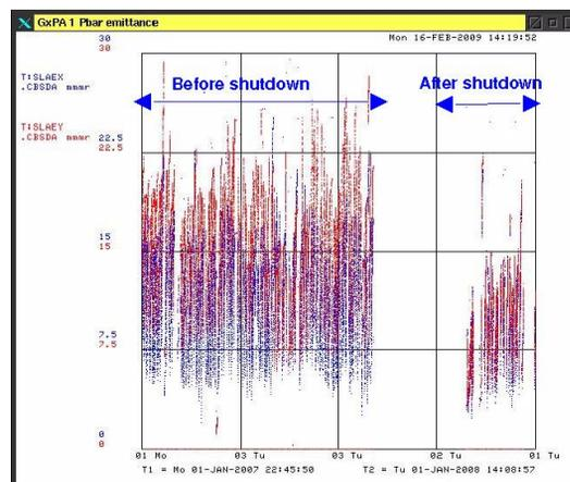
Figure 1: The average anti-proton emittance measured by the sync light monitor at collisions are shown here (T:SLAEX and T:SLAEY are the horizontal and vertical anti-proton emittances respectively). It is apparent that the anti-proton emittances are reduced after the 2007 fall shutdown. Note: the  $x$ -axis spans 1 year.
