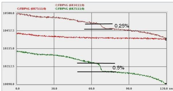
Figure 2: Store 6834 has a smaller loss during the transition from injection to collision helix compared to store 6825. The difference comes chiefly from the anti-protons which are larger by  $0.5\pi$  mm·mrad. For store 6875, the number of anti-protons at collisions is  $2\times$  smaller than stores 6825 and 6834, there is no loss through this transition. This clearly demonstrates that the source of the loss is from the beam-beam effect.
