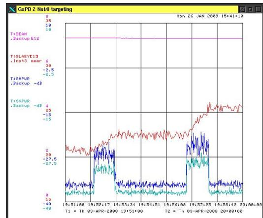
Figure 4: The transverse emittance of the anti-protons are blown up. T:SLAEY is the anti-proton vertical emittance. When the PBJ is turned on, the Schottky power (T:SHPWR and T:SVPWR) increases and the emittance increases. And when the PBJ is turned off the emittance remains constant.
