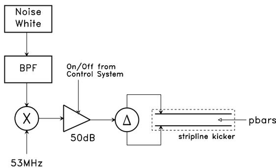
Figure 3: The PBJ kicks the anti-protons vertically. Both horizontal and vertical anti-proton emittances increase because of coupling although the beam is kicked vertically only.
