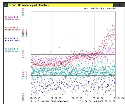
Figure 5: The horizontal and vertical transverse emittances of the protons (T:SLPEX and T:SLPEY respectively) are unaffected by the PBJ while the anti-proton emittances (T:SLAEX and T:SLAEY) are increased. Although the PBJ kicks the anti-protons vertically, there is horizontal emittance growth because of coupling.
