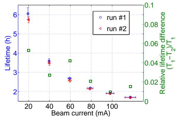
Figure 3: Lifetime as a function of the beam current for two different runs with the same beam conditions as in Fig. 2. The relative discrepancies of the measured lifetime of two runs are plotted using squares.
