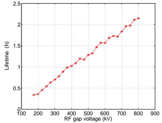
Figure 1: Lifetime as a function of the RF gap voltage. The storage ring is operated at 1.15 GeV with a 10 mA single-bunch beam.
