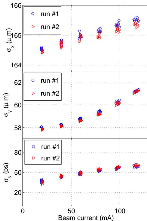
Figure 2: Transverse sizes and longitudinal bunch length of the electron beam as functions of the beam current for two different runs. The storage ring is operated at 1.15 GeV with 8 bunches. Top: the horizontal RMS beam size monitored by a synchrotron radiation profile monitor; Middle: the vertical RMS beam size; Bottom: the longitudinal RMS bunch length monitored by a dissector.
