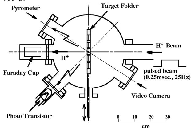
Figure 1: Experimental setup of a target chamber.
