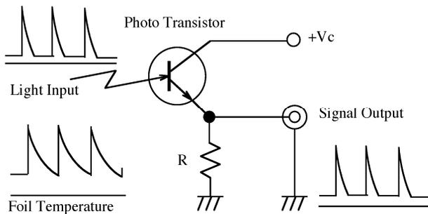
Figure 3: Electric circuit of photo detector
