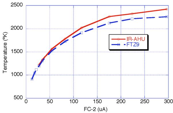
Figure 2: Brightness temperature on beam spot as a function of dc beam current during the irradiation.
