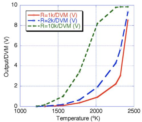
Figure 4: Photo-transistor output vs foil temperature by dc beams with R=1, 2, 10kΩ, respectively.
