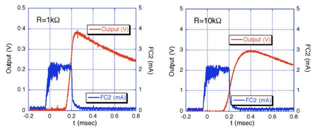
Figure 5: Beam pulses and output signals from a phototransistor by pulsed beam at various output resistors with R=1, 10 kΩ, respectively.
