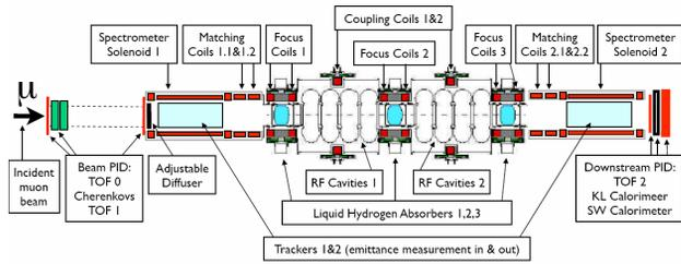
Figure 2: MICE cooling channel.
