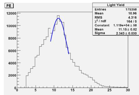
Figure 6: Light yield in first tracker determined using ~10,000 cosmic ray tracks.
