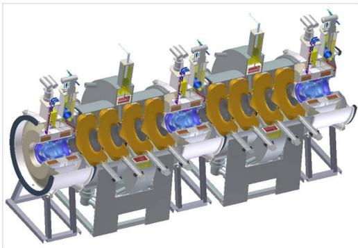
Figure 3: Full MICE cooling channel including three AFC modules and two RFCC modules.
