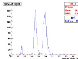
Figure 4: TOF distribution showing  $e^+$ ,  $\mu^+$  and  $\pi^+$  in a 300 MeV/c pion beam.
