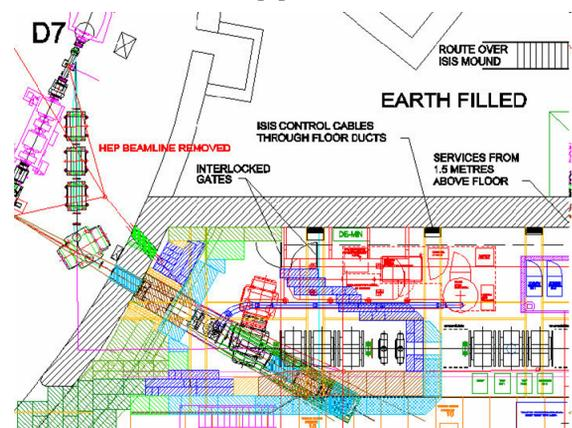
Figure 1: MICE beamline off the ISIS proton synchrotron at RAL.
