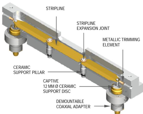
Figure 9: Planar test assembly / Cut-away view.
