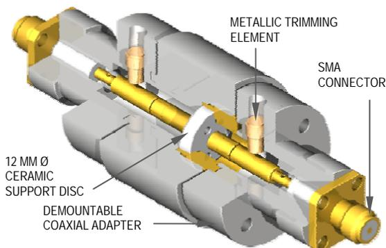
Figure 3: Coaxial Test Assembly / Cut-away view.
