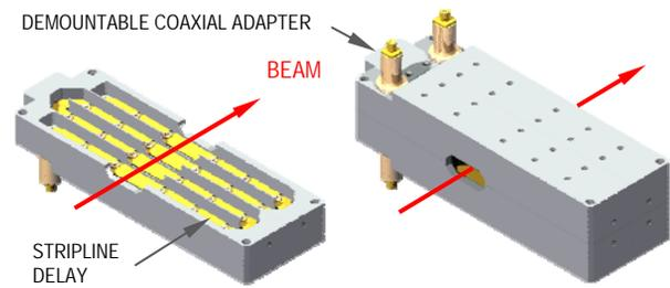
Figure 10: Short length planar prototype.
