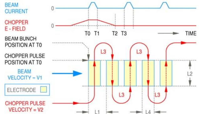
Figure 1: Slow-wave structure design.
