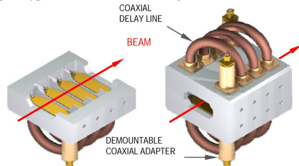
Figure 6: Short length helical prototype.
