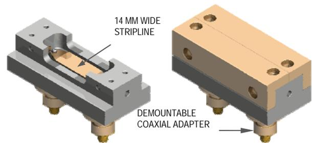
Figure 5: Helical Test Assembly.
