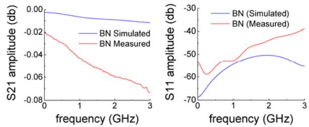
Figure 4: Coaxial Test Assembly / S parameters.
