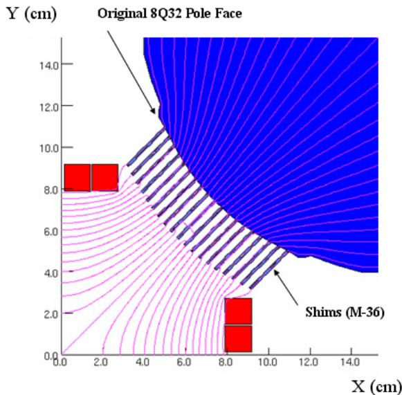
Figure 3: Modeled field with shims added.
