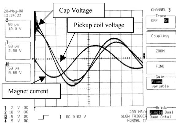
Figure 2: Ring Test showing response to impulse voltage.
