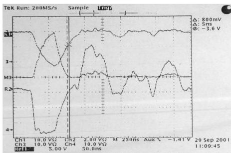
Figure 3: Voltage wave of the original Light II-A pulsed power generator by measurement (see the R2 curve).
