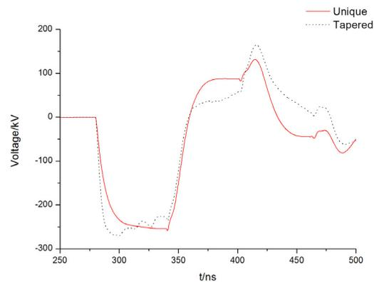
Figure 4: Voltage wave delivered by the new line on a 1.5Ω resistance (Solid: Unique impedance design; Dot: Tapered line design).
