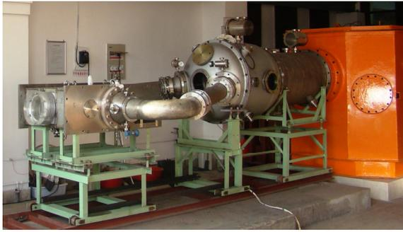
Figure 6: Installation of redesigned Marx generator and original experimental line.
