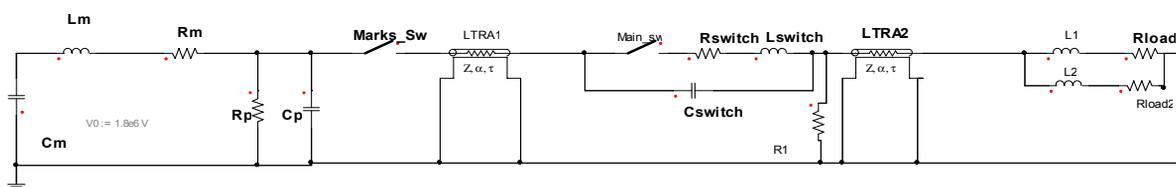
Figure 1: Circuit scheme of the original Light II-A pulsed power generator.
