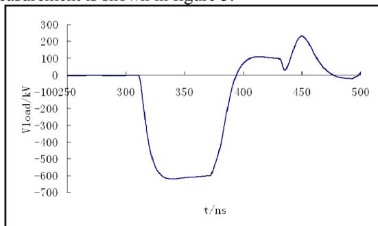
Figure 2: Voltage wave of the original Light II-A pulsed power generator by simulation.
