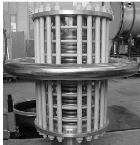
Figure 4: Laser triggered switch.
