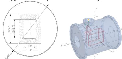
Figure 2: The structure of the prototype kicker magnet.
