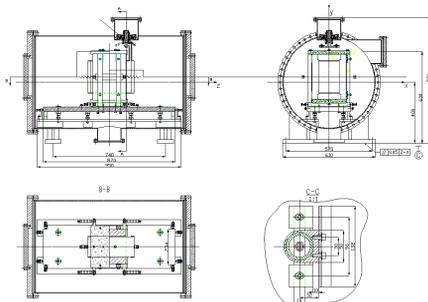
Figure 5: The drawing of the kicker magnet.
