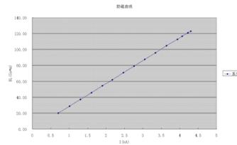
Figure 11: The relationship of the field and current.
