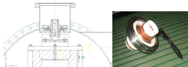
Figure 7: The high voltage feedthrough.
