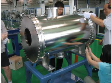
Figure 8: The assembly of the prototype magnet.
