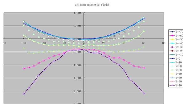
Figure 5: Integrated magnetic field distribution of the three-dimensional analysis.
