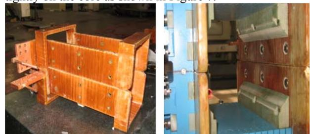
Fig. 7: The coil of the prototype BH magnet.
