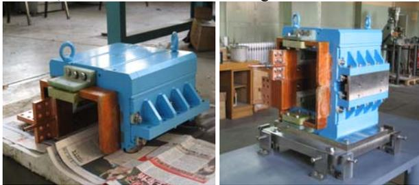
Figure 8: The assembly of the prototype BH magnet.
