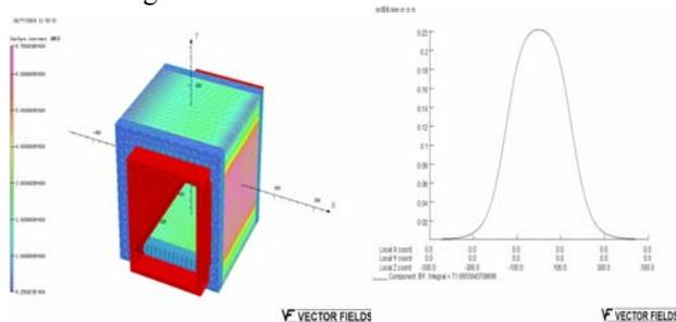
Figure 4: The OPERA-3D simulation.
