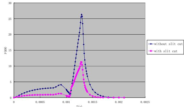
Figure 6: Calculated results of the eddy current losses.
