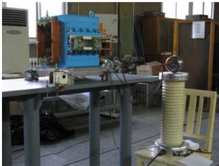
Figure 10: The electric withstanding voltage test.
