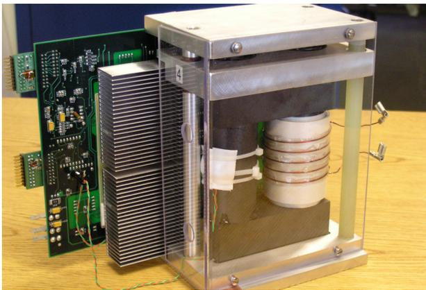
Figure 3: H-bridge driver and transformer module assembly.
