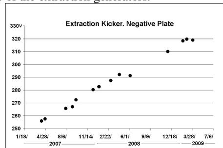
Figure 1. DC voltage on the pre-ionization electrode.
