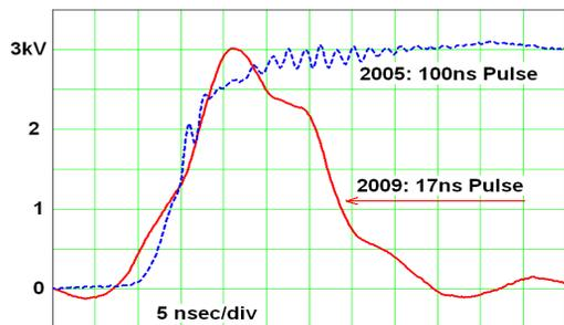
Figure 3. Evolution of the injection pulse front edge.
