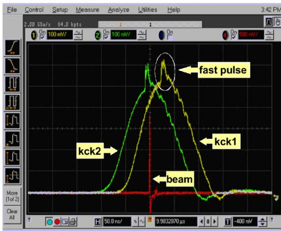
Figure 4: “Hybrid” injection: long and fast pulses, from two striplines of e+ ring kickers, observed in sum at the scope.
