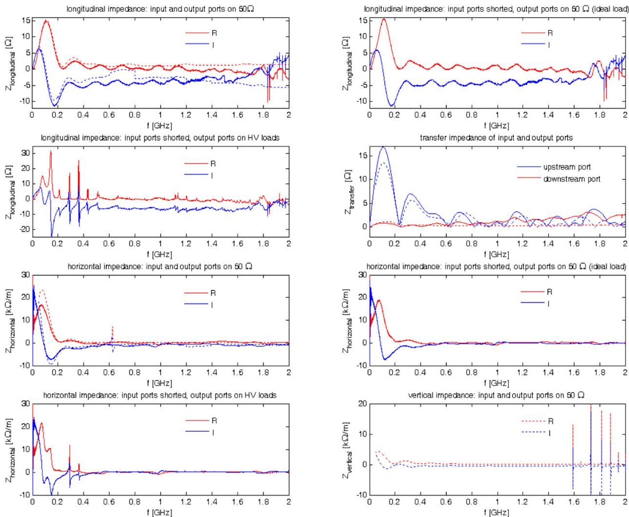
Figure 3: results of impedance measurements (solid lines) and simulations (dashed lines).
