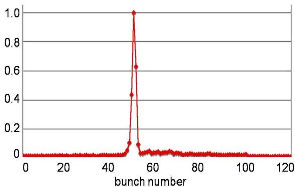
Figure 5: 100, of 120, stored bunch r.m.s. oscillation amplitude with kicker pulse centred on bunch 50.
