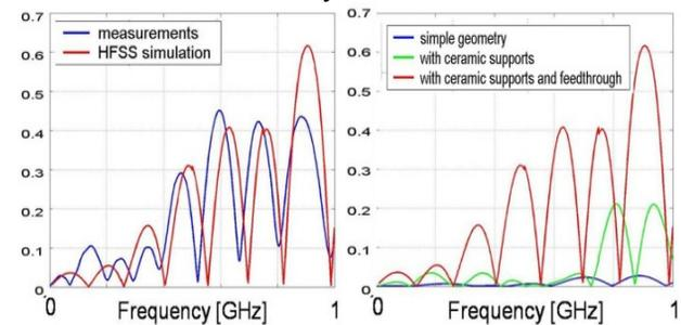
Figure 2: Reflection coefficient ( $S_{11}$ ) at the input port.
