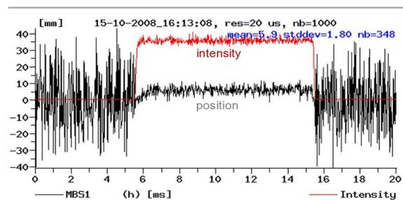
Figure 2: A beam position measurement during a UCN full-intensity short kick. The beam deflection by the kicker magnet can clearly be seen during the first 2 ms of the kick. The measurement of the beam intensity is superposed to the beam position. At zero beam intensity, the position measurement is meaningless.
