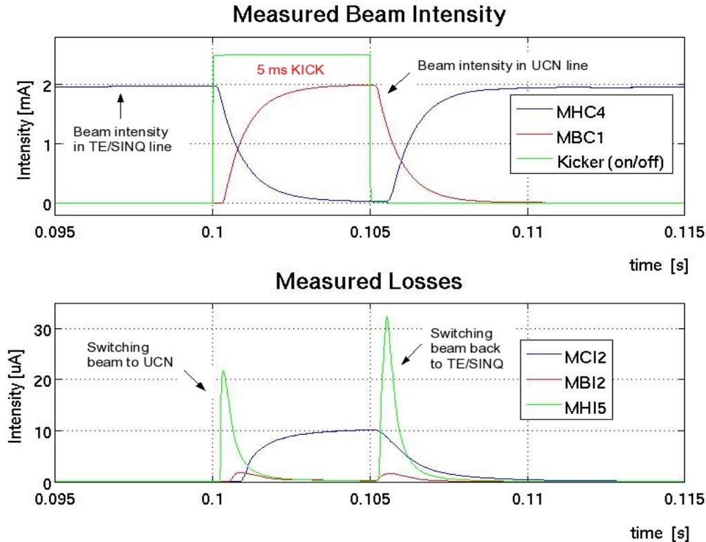
Figure 3: Measurements of beam intensity and losses during a 5 ms UCN kick at full intensity. The three loss monitors are only a subset of the several ionization chambers employed in the line. Their positions are shown in Fig. 1.
