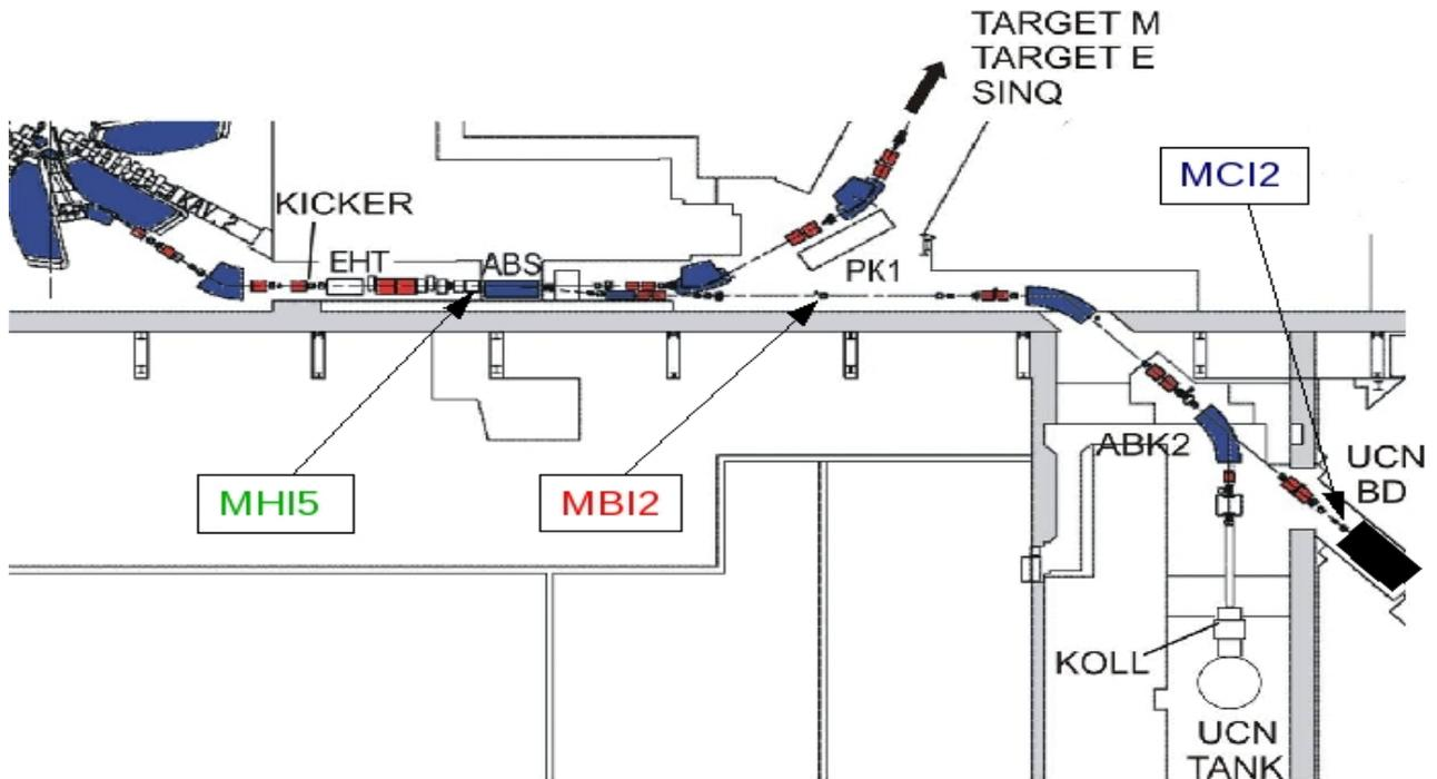
Figure 1: A schematic view of the UCN beam line. The different components are described in the text. MHI5, MBI2 and MCI2 are the three beam loss monitors whose measurements are shown in Fig. 3.
