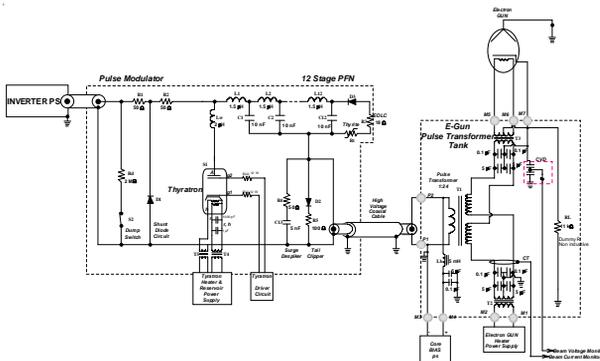
Figure 3: Line type pulse modulator schematic diagram.
