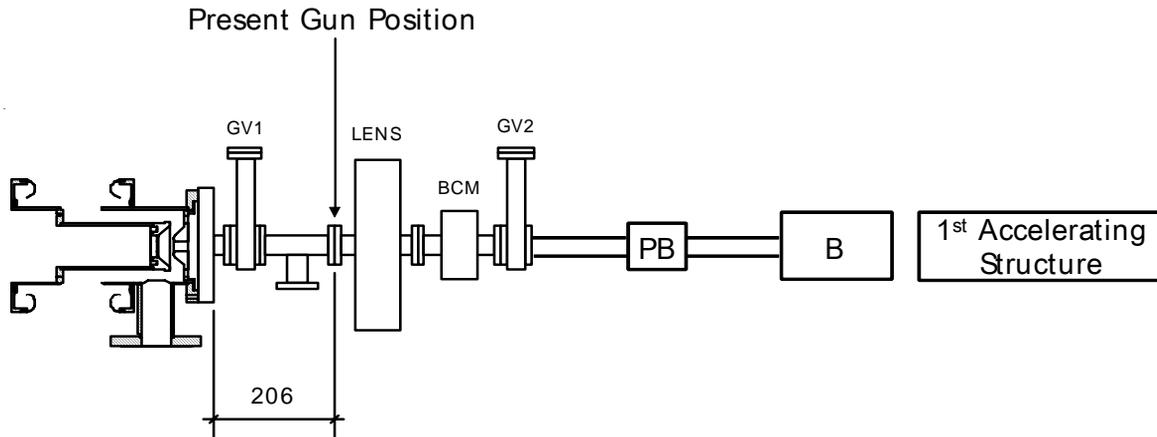
Figure 1: Layout of the PLS-II Electron Gun. For fast replacement of the gun on gun failure, a spare gun with a gate valve attached is prepared at fully operational condition, moved to the accelerator tunnel with the gate valve attached to it, and installed to beam line.
