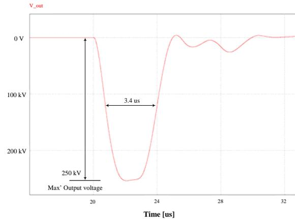
Figure 4: Output voltage waveform.
