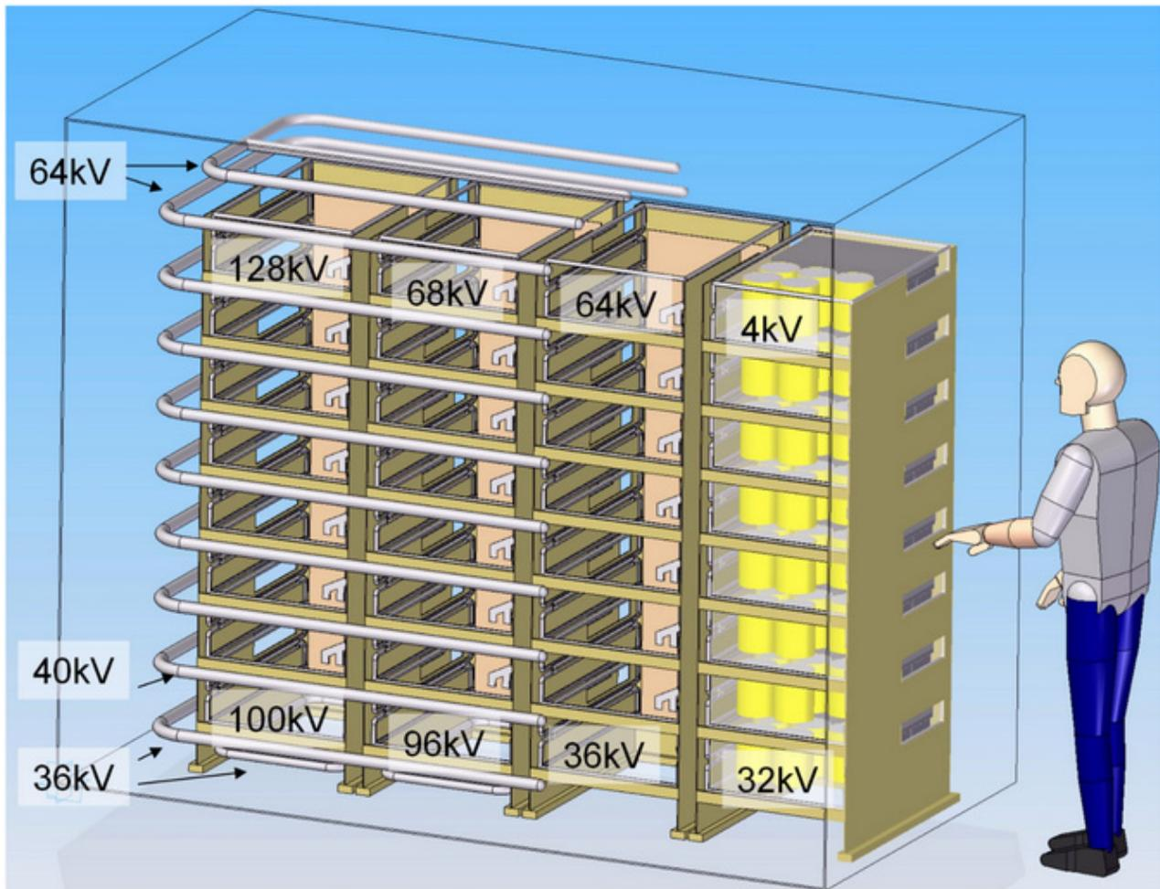
Figure 4. Conceptual design of the P2 Marx.
