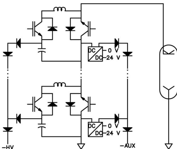
Figure 1. Simplified schematic of the ILC Marx.
