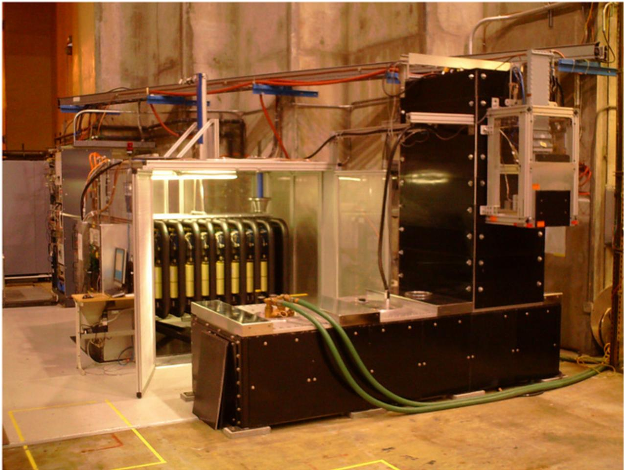
Figure 3. L-band test station; 10 MW klystron (right), Marx modulator (center), Rf controls (left).
