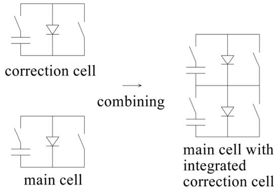
Figure 2: Schematic representation of the proposed droop correction concept. Both cells consist of an energy storage capacitor, a charge switch (right switch), a discharge switch (left switch) and a bypass diode.
