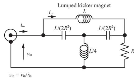
Figure 1: Proposed kicker system: Bridged-T network lumped kicker.
