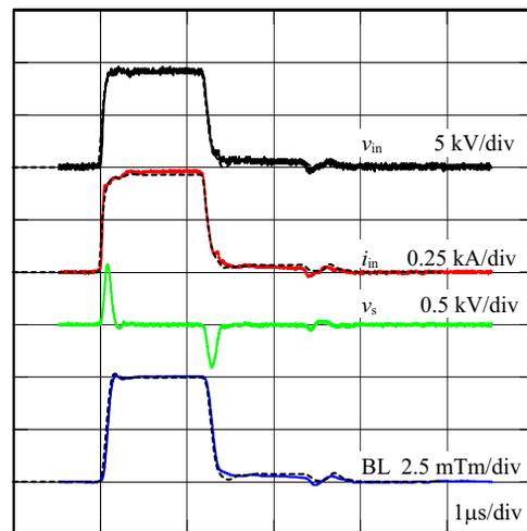
Figure 3: Pulse response. The dashed lines show calculations from a SPICE simulation.
