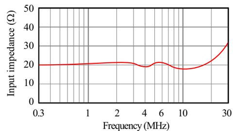
Figure 4: Input impedance.
