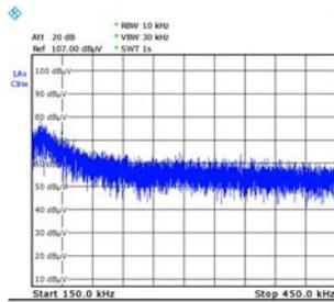
Figure 10: Noise spectrum matches FCC Class A Part 15 standard second section.
