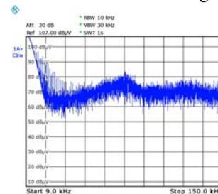
Figure 9: Noise spectrum can't pass FCC Class A Part 15 standard first section without filter.
