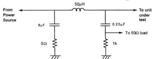
Figure 5: Indicates the LISN component of decomposed diagram.
