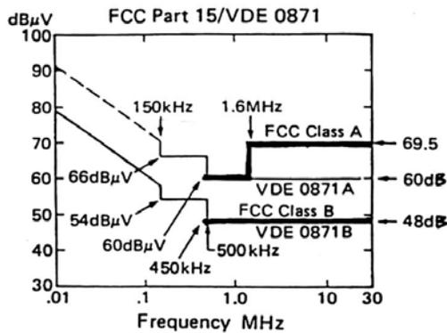
Figure 4: FCC Part 15 and VDE 0871 with frequency diagram.
