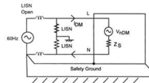
Figure 7: The differential mode current path IDM
