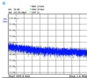
Figure 11: Noise spectrum matches FCC Class A Part 15 standard 3rd section.
