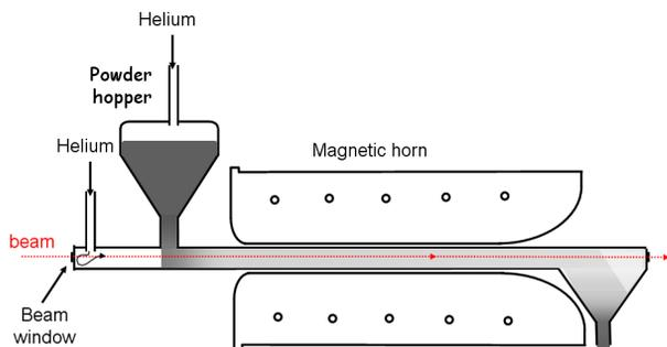
Figure 1: Illustration of contained flowing powder target.
