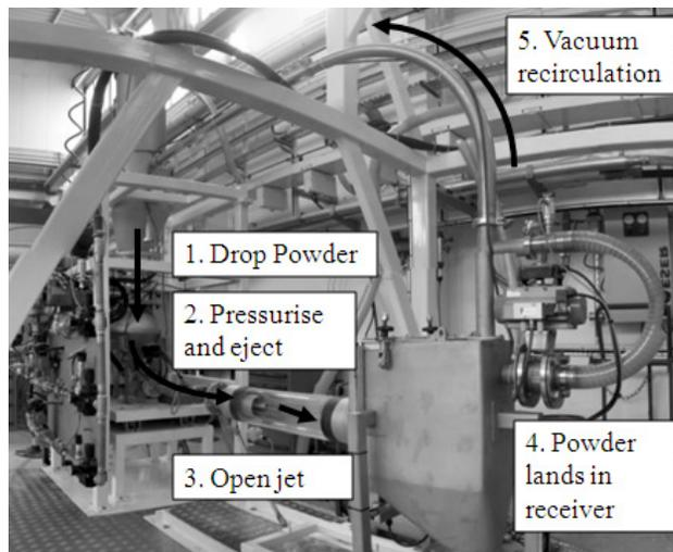
Figure 3: Powder handling test rig at RAL.
