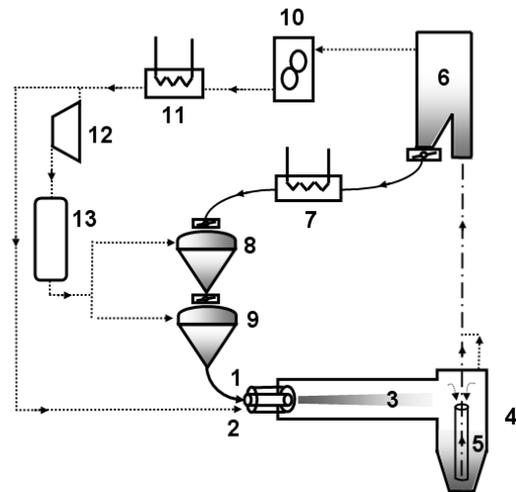
Figure 2: Schematic outline of a circuit for continuous powder target supply, with (1) powder discharge nozzle, (2) gas return line forming coaxial flow, (3) either open target jet (shown), or flow within pipe (4) receiver hopper, (5) suction nozzle for gas lift, (6) gas lift receiver vessel with filter, (7) powder heat exchanger, (8) and (9) pressurised powder hoppers, (10) Roots blower, (11) gas heat exchanger, (12) compressor, and (13) gas reservoir.
