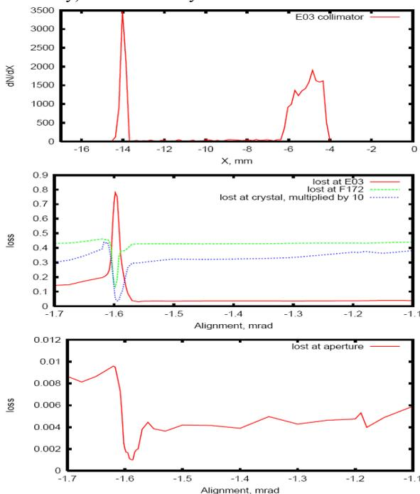
Figure 5: Channeled and partially channeled peaks at E03 (top), fractional beam loss on E03 and F172 collimators and crystal (middle), and fractional beam loss in the rest of the Tevatron (bottom), for miscut angle  $\theta_m = -1.6 \text{ mrad}$ .
