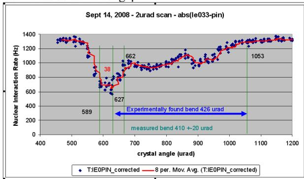
Figure 2: Results of crystal angular scan.
