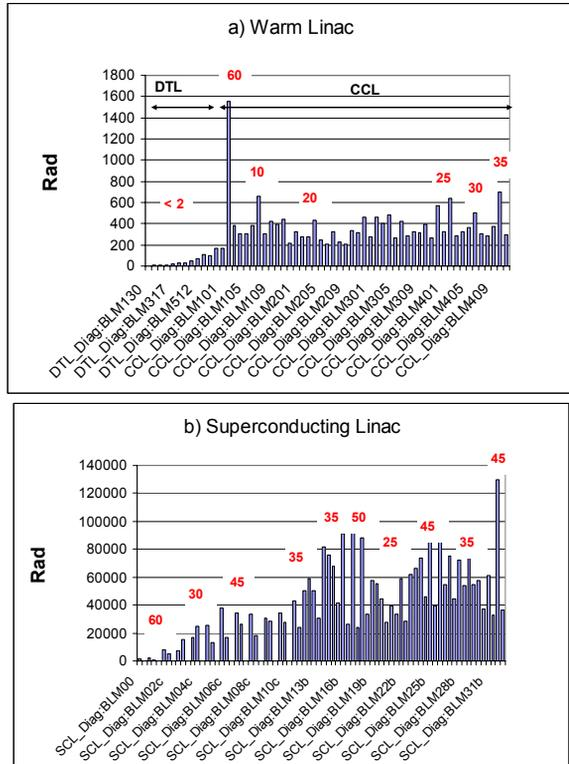
Figure 2: Beam loss throughout the a) warm linac and b) SCL. Numbers in red are residual activation levels after a 16-day production run at 730 kW.
