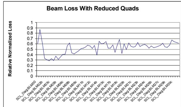
Figure 3: Ratio of beam loss with reduced focusing strength to beam loss with design quadrupole strength in the SCL.
