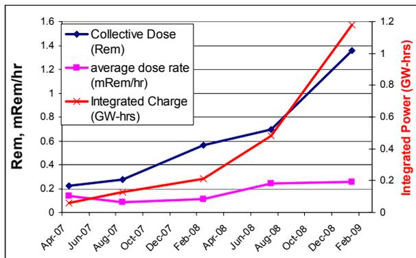
Figure 7: Worker dose accumulation during maintenance periods following major run cycles, along with the integrated power delivered during the run-cycle.
