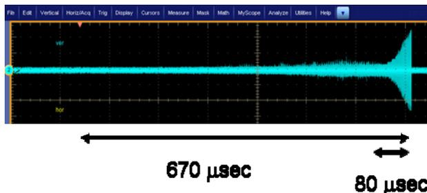
Figure 10: Vertical difference signal in the Ring indicating possible e-p activity near the last 80  $\mu\text{sec}$  of a 670  $\mu\text{sec}$  beam accumulation during neutron production.
