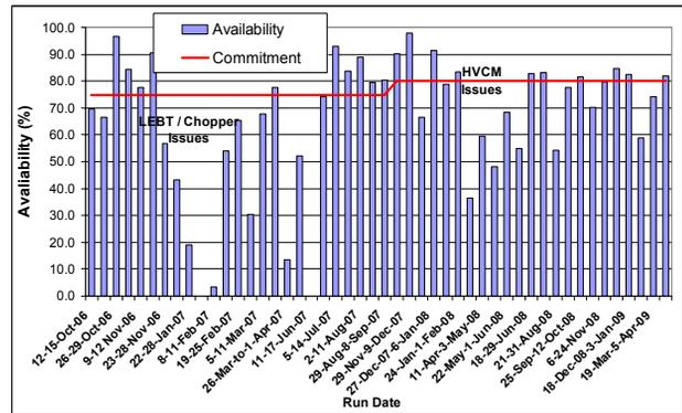
Figure 8: Beam availability (= actual on time / promised on time) since the start of beam operations at SNS.
