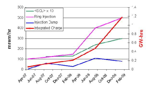
Figure 5: Build-up of residual activation levels following major run cycles, and the increase in the integrated power delivered to the Target. Green is the average SCL warm section activation, pink is the Ring injection area and the blue line is the Injection dump-line activation
