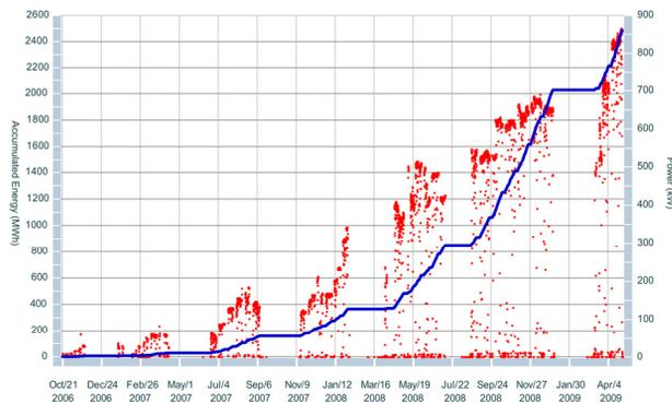
Figure 1: Progress in ramp up of the beam power since the start of operations (Beam power in red and integrated charge delivered in blue).
