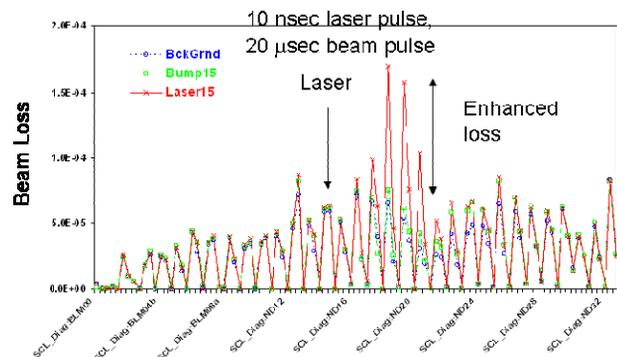
Figure 6: Beam Loss in the SCL with (red) and without (green) a diagnostic laser on, used as a method to calibrate the loss signal to a know amount of beam.
