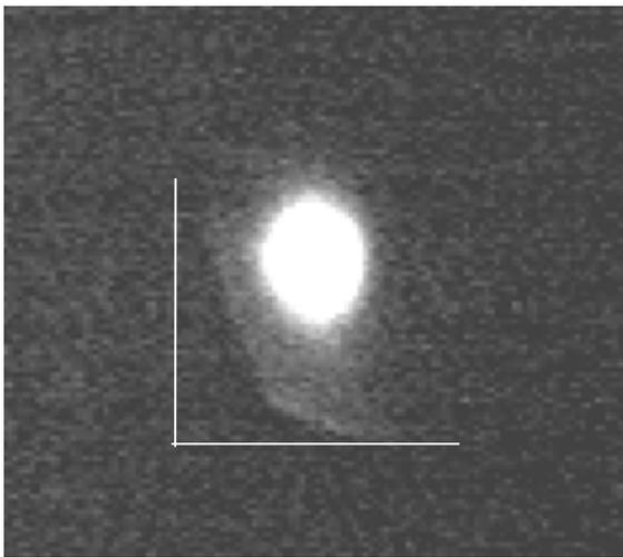
Figure 9: Image of the SNS Stripper foil under 860 kW beam operations with an outline inserted indicating the original corner position.
