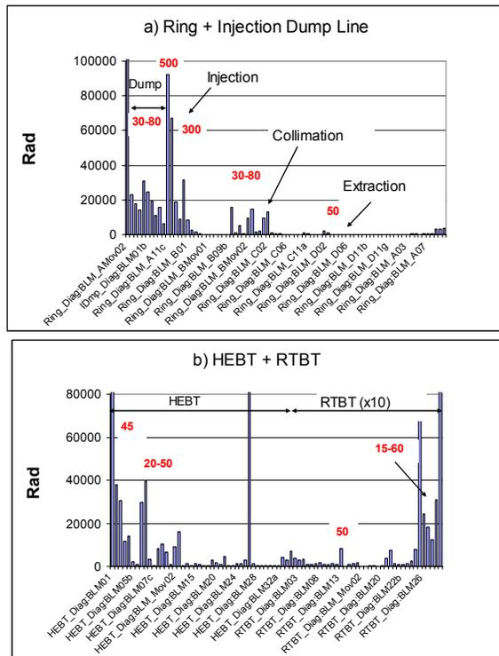
Figure 4: Beam loss and residual activation a) in the Ring and Ring injection dump line and b) in the transport lines for the same case as Figure 2.
