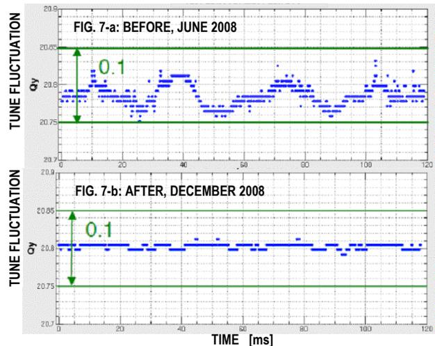
Figure 7: Tune fluctuation before (upper) and after the wiring re-configuration (lower) are shown.
