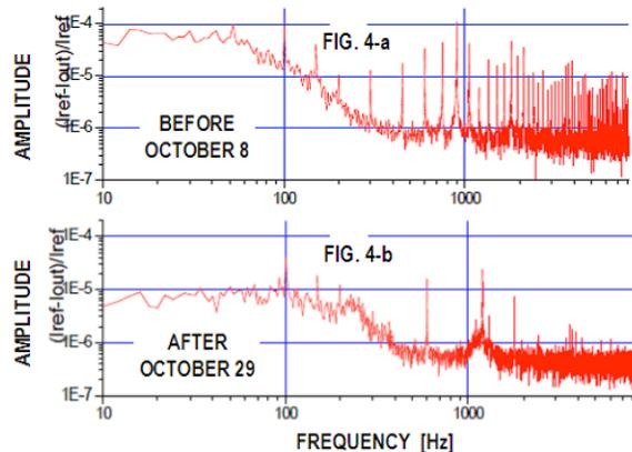
Figure 4: Subtraction of two current monitors. The original situation with unsymmetrical cabling (a). After the re-configuration of the cabling network (b).
