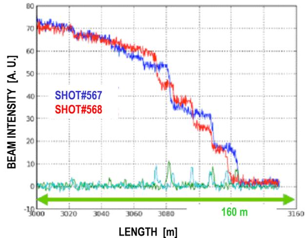
Figure 15: Beam current during extraction. The two decaying lines record the stored current in the MR for two arbitrary shots. Corresponding impulsive extracted beam currents are shown in the bottom trace.
