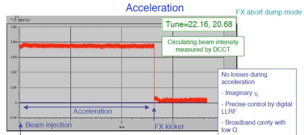
Figure 10: Beam current during acceleration. Acceleration time was 2.5 sec, then beam was extracted by the fast extraction system.
