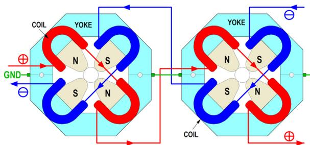
Figure 5: Quadrupole magnet connections. Like polarity poles are series connected.
