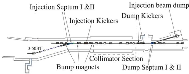
Figure 8: Layout of the injection and collimator section.
