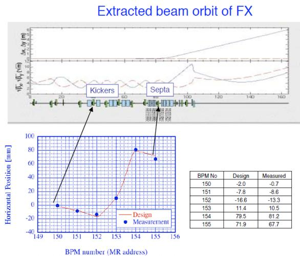
Figure 14: Schematic view of the fast extraction section (upper). Horizontal beam position along extraction section (lower): measured (dots) and designed (line).
