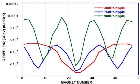
Figure 2: Quadrupole field-components measured along the tunnel at 300 Hz, 750 Hz and 900 Hz.
