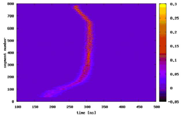
Figure 11: Longitudinal beam profile during acceleration. Vertical: acceleration time from 0 to 2.5 sec. Horizontal: relative phase between beam and accelerating microwave (full width 500 nsec).
