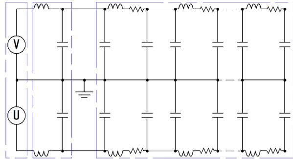
Figure 3: A symmetrical power supply and cabling configuration as described in ref. [2].
