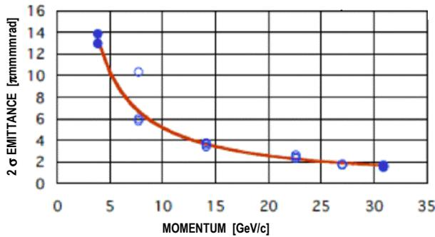
Figure 13: Measured beam emittance from 3 GeV to 30 GeV (circles). The line shows emittance as a function of beam momentum.
