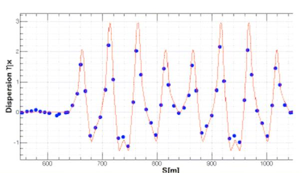
Figure 12: Measured dispersion (blue dots) shown with the design calculated plot (red line).
