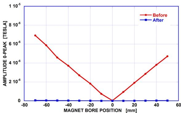
Figure 6: Quadrupole field-components measured at 900 Hz (common mode frequency). Plots are from before and after cabling re-configuration.
