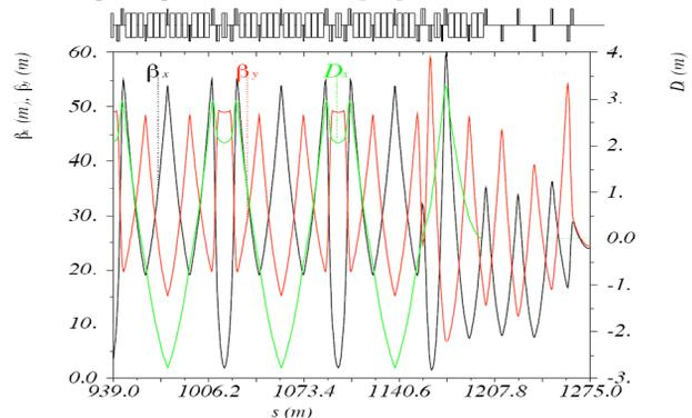
Figure 3: Optical functions for a quarter of the PS2 ring.
