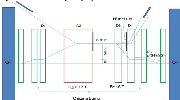
Figure 5: H Injection. The first chicane dipole (red) has low field  $B \leq 0.13$  T to avoid Lorentz stripping of the incoming H. Kickers (green) make the painting bump.
