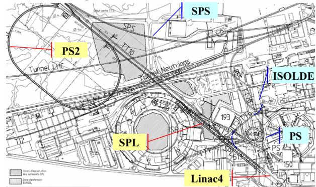
Figure 2: Integration of PS2 within the existing and future CERN accelerator complex.
