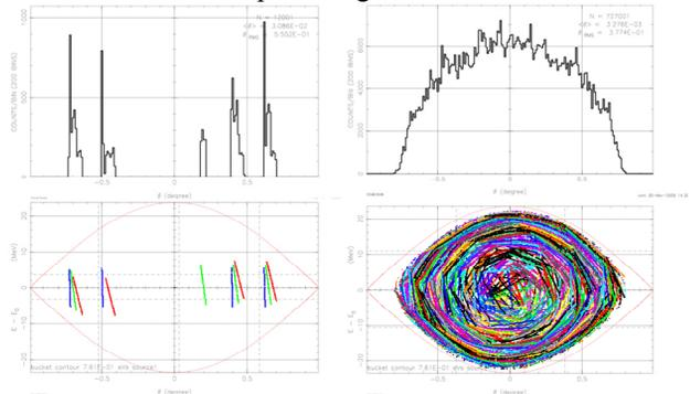
Figure 6: Longitudinal painting with a complex chopping scheme to depopulate the central phase space region [25].
