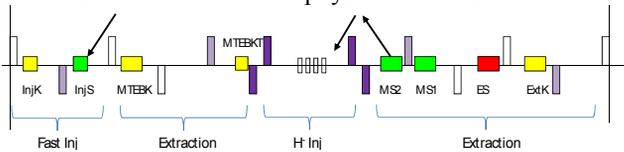
Figure 4: Layout of injection and extraction elements in the long straight section. (MS1, MS2 magnetic septa, ES electrostatic septum, ExtK: fast extraction kicker, MTEBK(T): fast kickers to close 5-turn extraction bump, InjS: ion injection septum, InjK: ion injection kicker).
