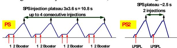
Figure 7: LHC cycle in SPS with PS and PS2 as injector.
