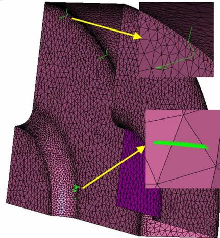
Figure 10: MPs trajectories at 1.3 MV/m peak surf. field.
