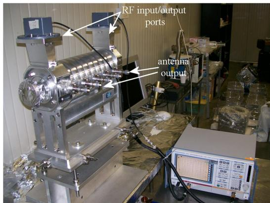
Figure 4: RFD under test
