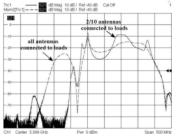
Figure 6: Transmission coefficient between two antennas
