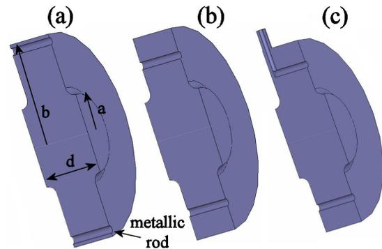
Figure 1: Single cell geometry: (a) old; (b) rod modified; (c) rod modified and damping antenna.
