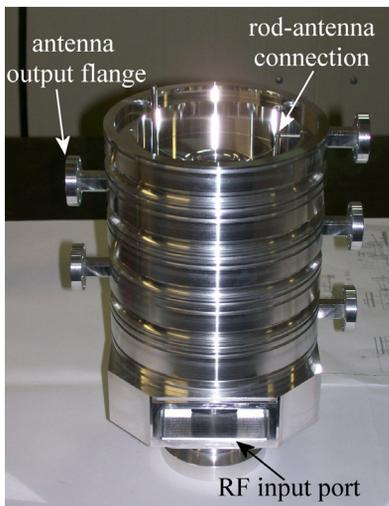
Figure 3: Assembled RFD cells.
