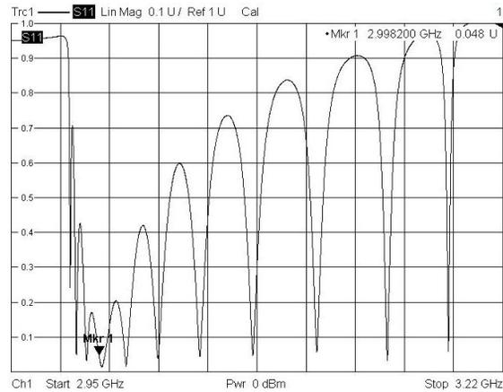
Figure 5: Measured reflection coefficient at the input port
